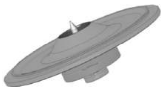
Figure 2-17: Lid of an aerosol-tight rotor with mandrel
