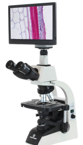
3013-LED with HDS Lite camera (Camera/monitor and C-mount sold separately)
