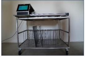
The Automatic Layer Thickness Measurement machine (ALTM) can produce accurate and reproducible pattern measurements on applied coated panels. This device is used in the paint and coating industries to determine the layer thickness variations on a substrate in order to determine thickness fluctuations and thus optimise the application process.
