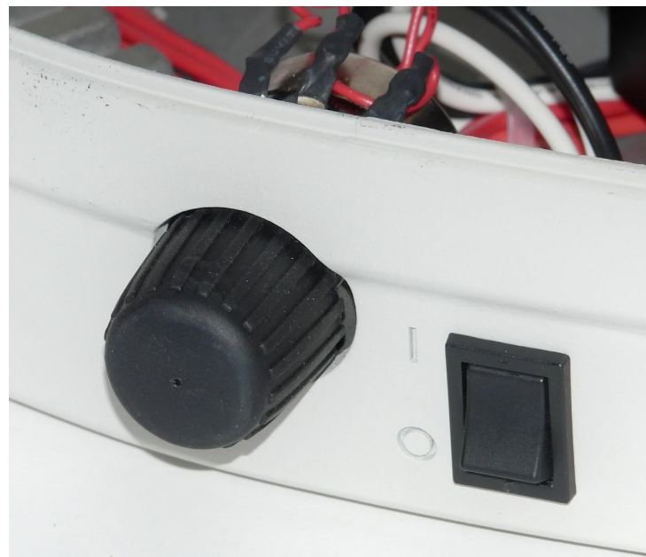
(1) The rubber cover must be removed from the knob. It is glued to the knob, and extends past the inside edge of the knob, making it difficult to remove.
