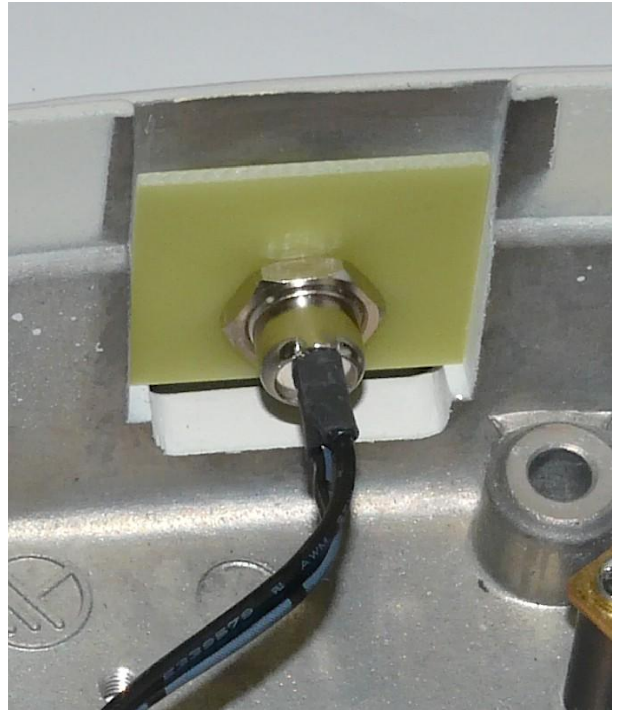
(4) Verify that both plates are properly aligned with the nut finger tight. Then finish tightening with a wrench, just enough to secure them. Don't over-do it.
