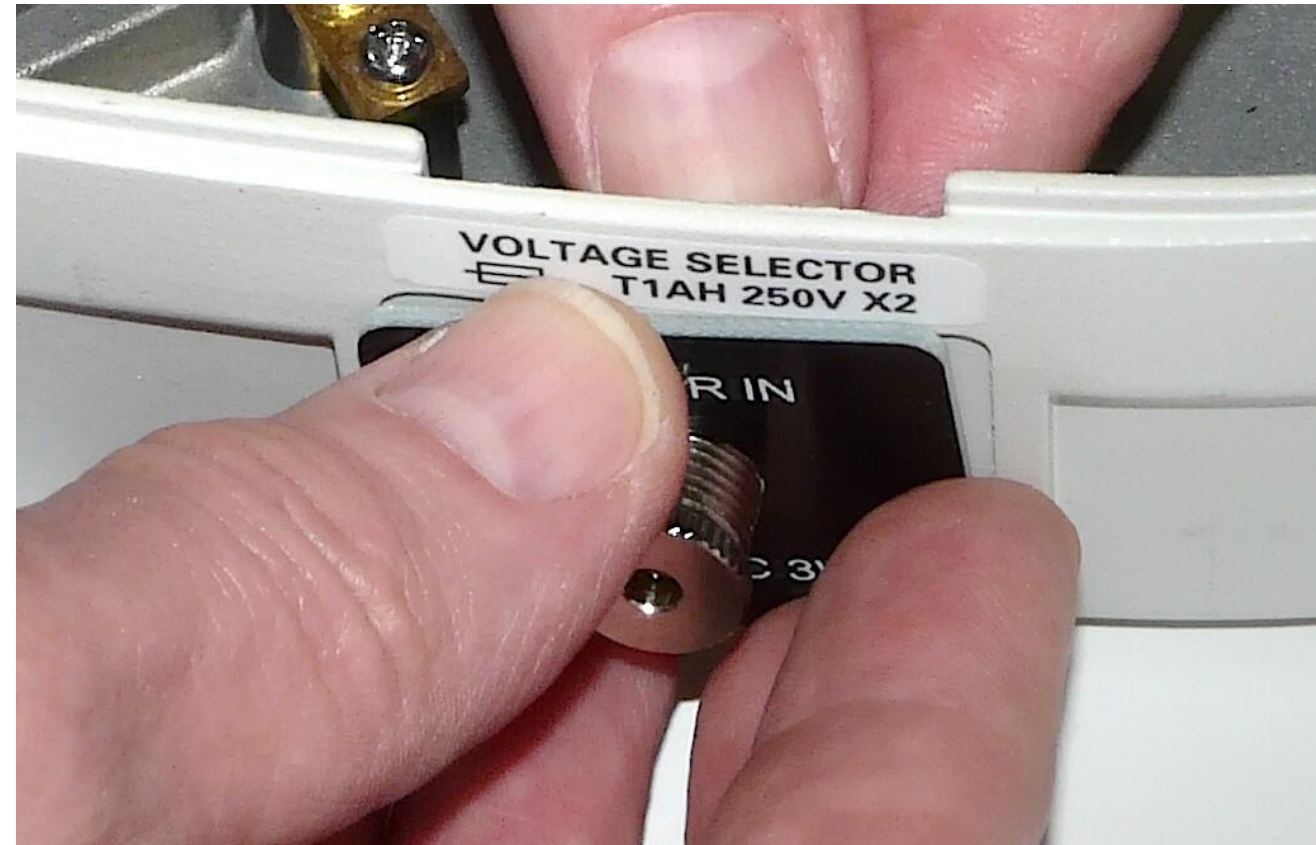
(3) Line up the power plate (on the outside), and the retainer plate (on the inside) with the recesses in the microscope frame. Then thread the nut onto the silver metal power jack and tighten it by hand.
