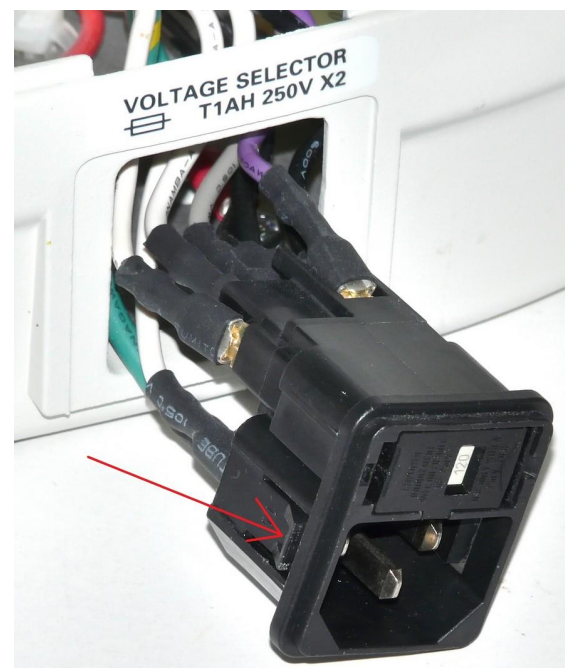
(6) Depress the plastic clips on each side of the AC power receptacle and push it out.
