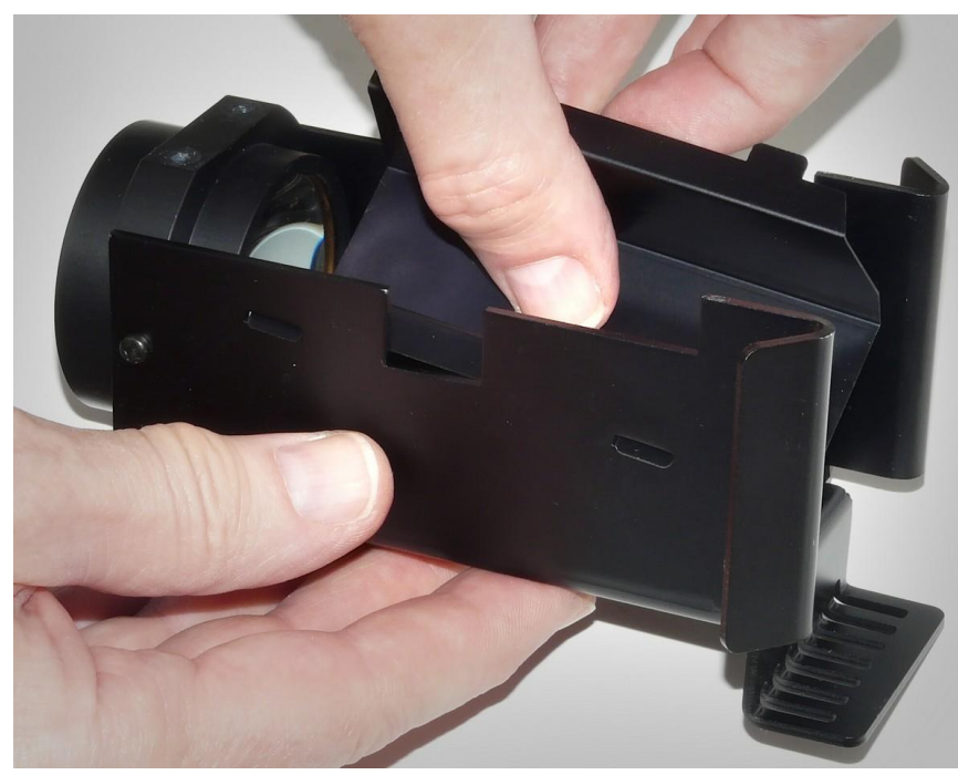
(3) Remove the heat shield from the collector lens/lamp housing assembly. (it interferes with the power cable on the new assembly)
