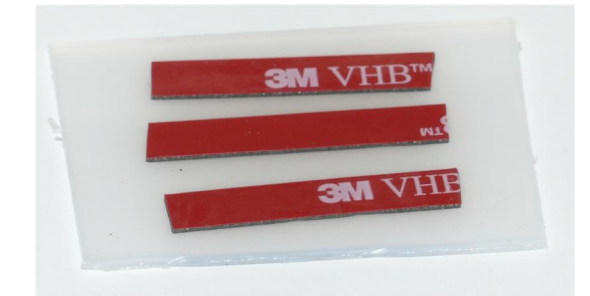
Tape to secure wires.
