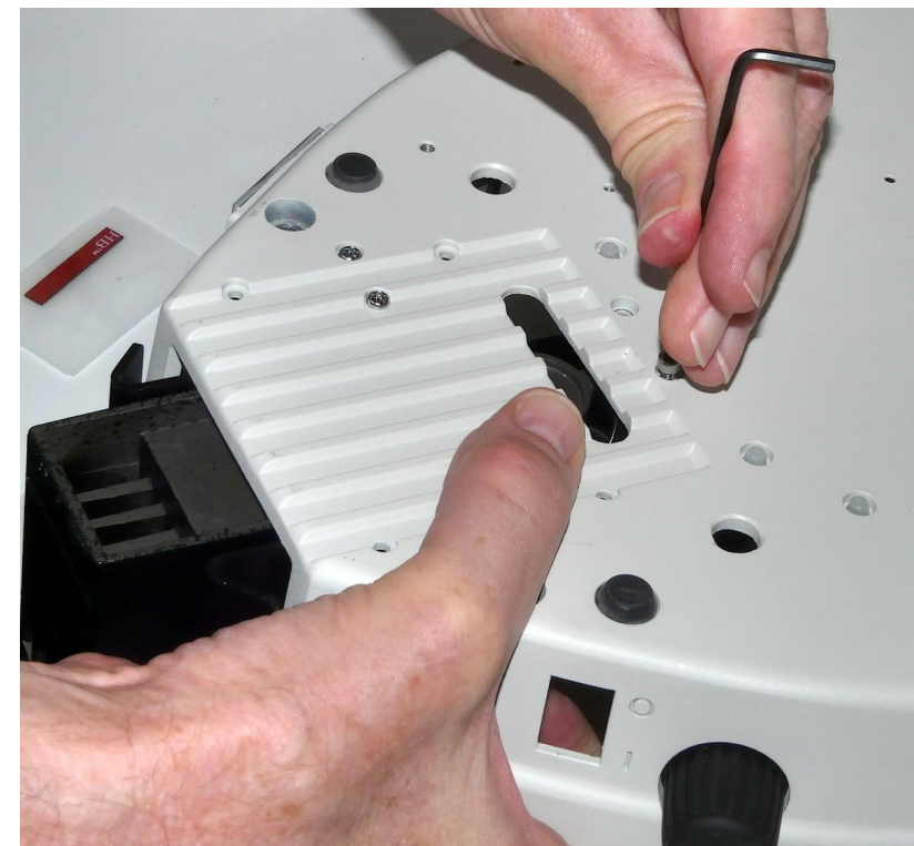
(4) Attach the lamp housing as it was removed, using the original screws.
