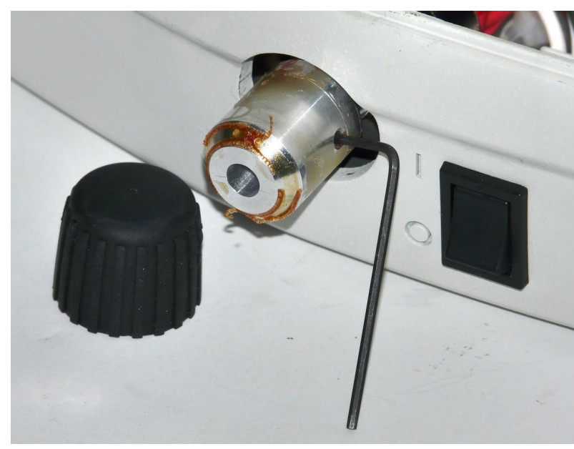
(3) Pull or push the rubber cover off the knob. Then loosen the set screw to remove the knob.
