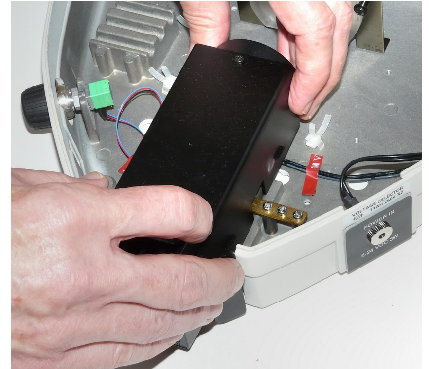
(3) Replace the collector lens/lamp housing assembly
