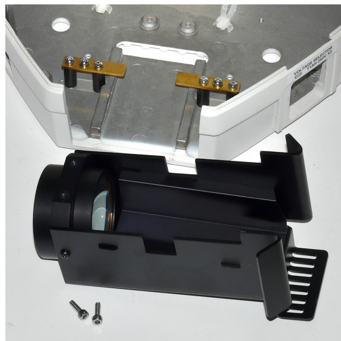
(2) Remove the collector lens/lamp housing assembly. (it interferes with the power cable on the new assembly)
