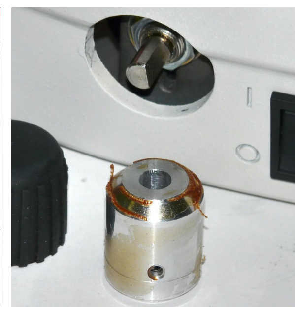
(4) Knob removed from potentiometer. Keep both knob and rubber cover to install on replacement potentiometer.
