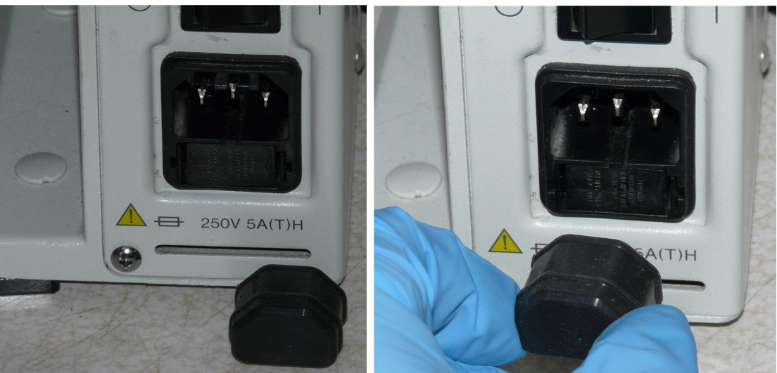
(2) Install PN 10736 rubber plug in AC receptacle to deter connection of AC power.
