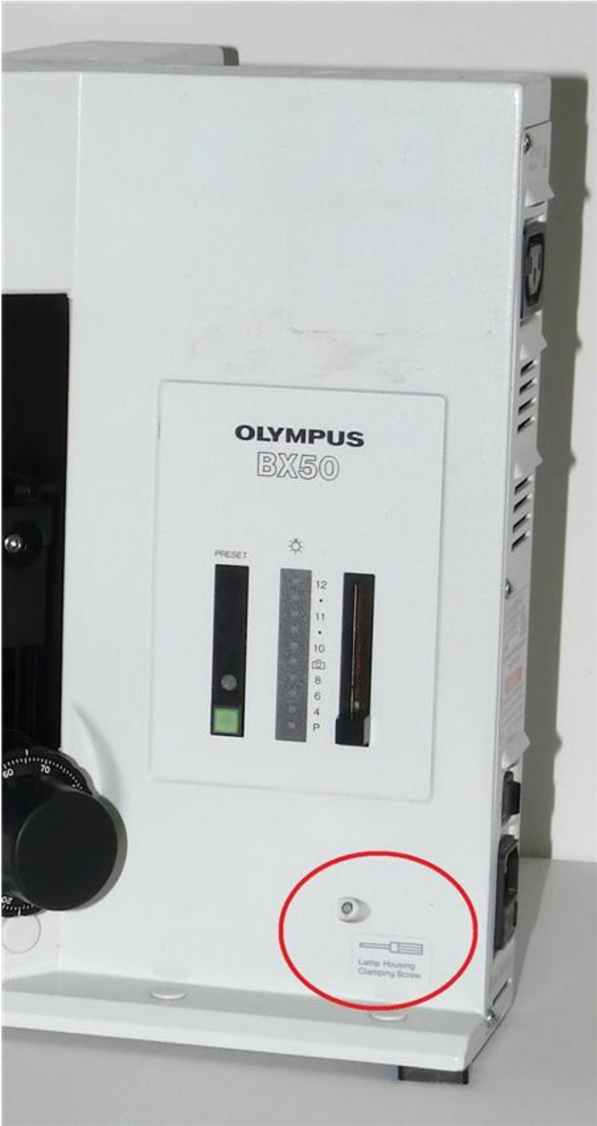
(1) Use the tool recessed in the top of the microscope to release the illuminator.
