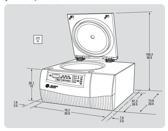
Figure A.1 Centrifuge Dimensions
