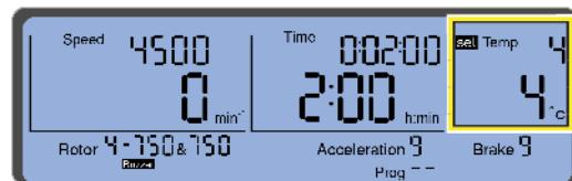
**NOTE** To reach temperatures above ambient, the centrifuge is dependent on the frictional heat generated inside the chamber during operation. At low run speeds or low ambient temperatures, the centrifuge may not be able to achieve some higher temperatures.
