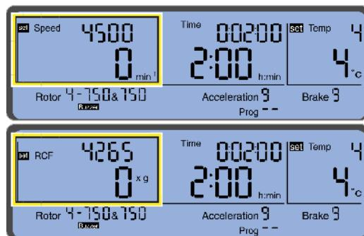
The parameters speed and RCF can be changed during the centrifugation run.
