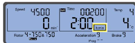
The time parameter can be changed during the centrifugation.
