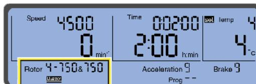
3 Navigate to **Buzzer** again (if necessary) and press the **ENTER** button to deactivate the Buzzer function. In this case, the Buzzer symbol disappears but the bar that was underneath the symbol will continue to flash.
