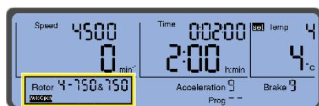
3 Navigate to **AutoOpen** again (if necessary) and press the **ENTER** button to deactivate the “Auto Open” function. In this case, the AutoOpen symbol disappears but the bar that was underneath the symbol will continue to flash.
