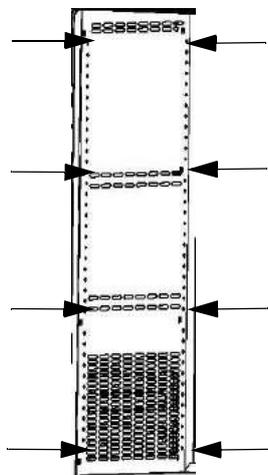
**Figure 5-7 Removing the left and right support profiles**
