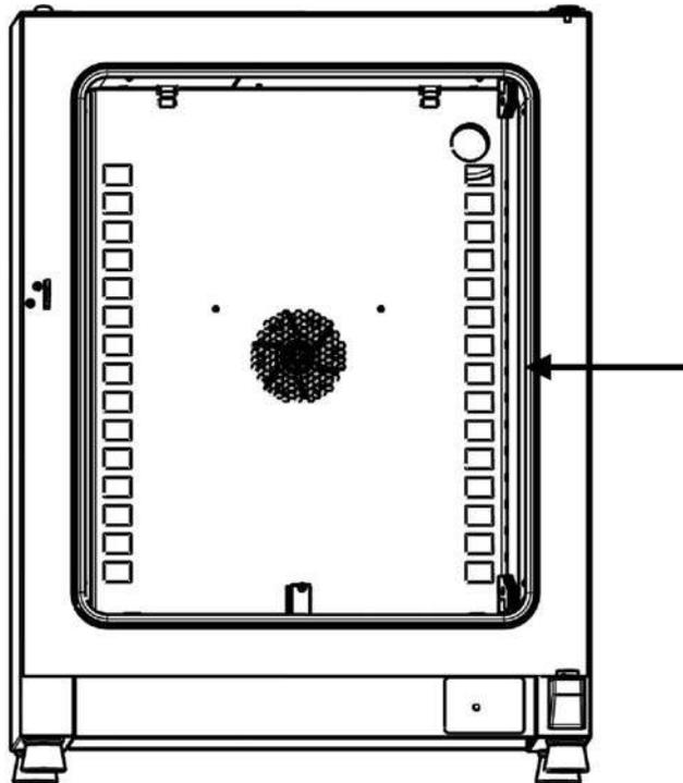
**Figure 10-1 Door Seal Replacement**
