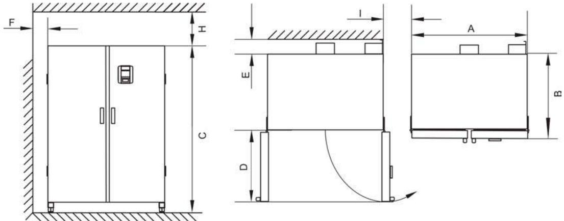
Figure 3-3 Floor Stand Incubators, dimensions and required clearances
