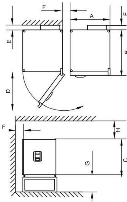
**Figure 3-1 Table-top Incubators, dimensions and required clearances**
