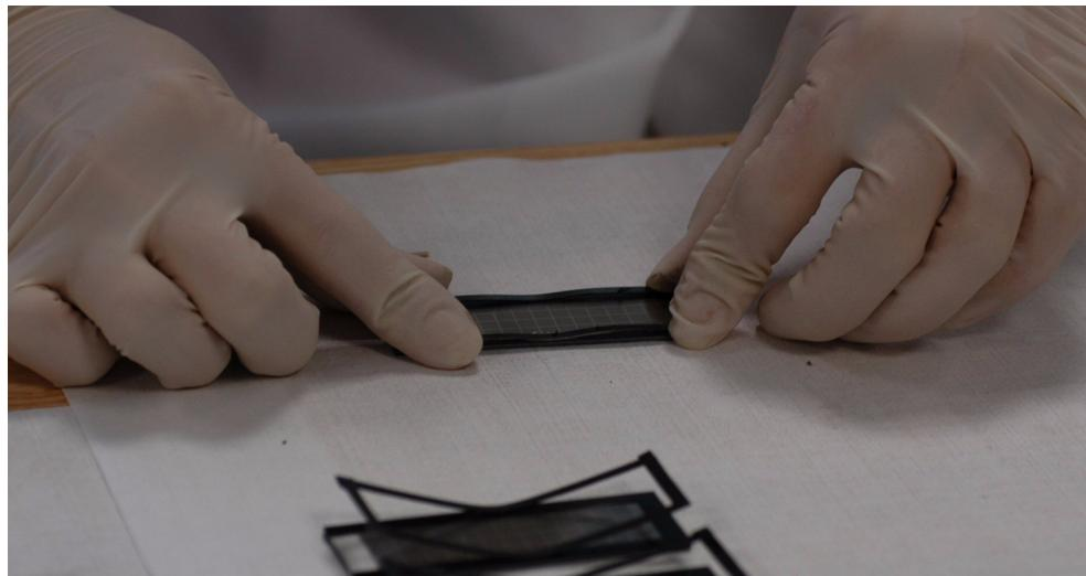
The OpenArray plate is now sealed, framed, and ready to insert in the OpenArray NT Cycler.
