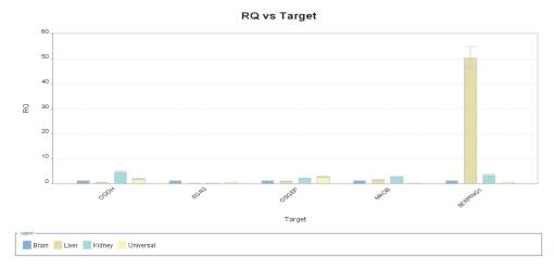
• **RQ vs Sample** – Groups the relative quantitation (RQ) values by sample. Each target is plotted for each sample. You can display the plot on a linear, log10, Ln, or log2 scale.
