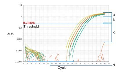
**IMPORTANT!** Experimental error (such as contamination or pipetting errors) can produce atypical amplification curves that can result in incorrect baseline and threshold value calculations by the 7500 software. Therefore, Applied Biosystems recommends that you examine the Amplification Plot screen and review the assigned baseline and threshold values for each well after analysis is complete.
