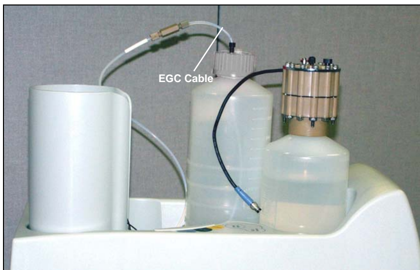
Figure 43. Dionex EluGen Cartridge in Service Area
