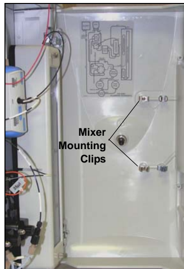
Figure 93. Location of Mounting Clips for the Dionex EGC CO 3 Mixer
