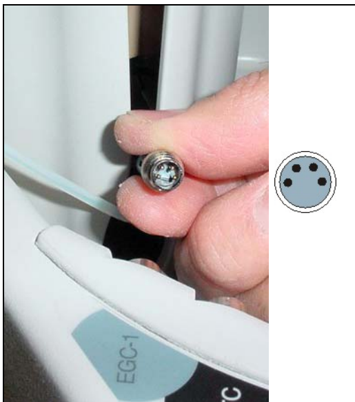
Figure 47. Connecting the Dionex EluGen Cartridge Cable
