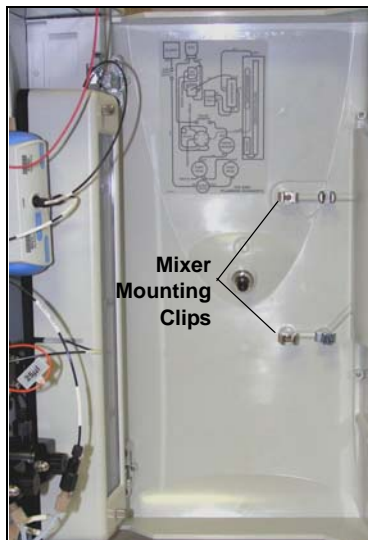
Figure 73. Location of Mounting Clips for the Dionex EGC CO 3 Mixer
