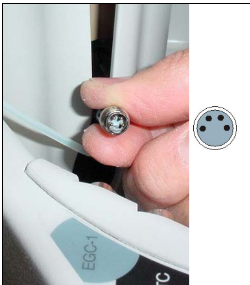
Figure 63. Connecting the Dionex EluGen Cartridge Cable
