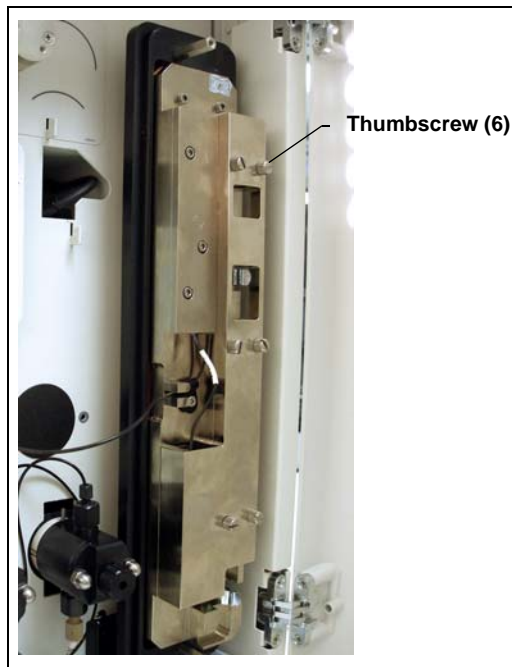
Figure 27. Column Heater with Cover Removed
