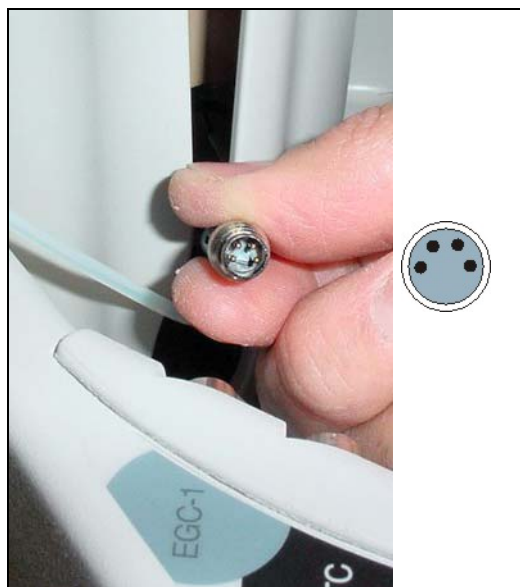
Figure 87. Connecting the Dionex EluGen Cartridge Cable
