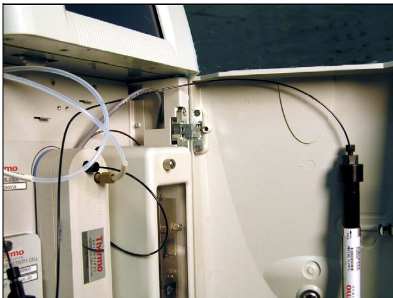
Figure 80. Mixer Outlet Routed to the Back of the Component Panel
