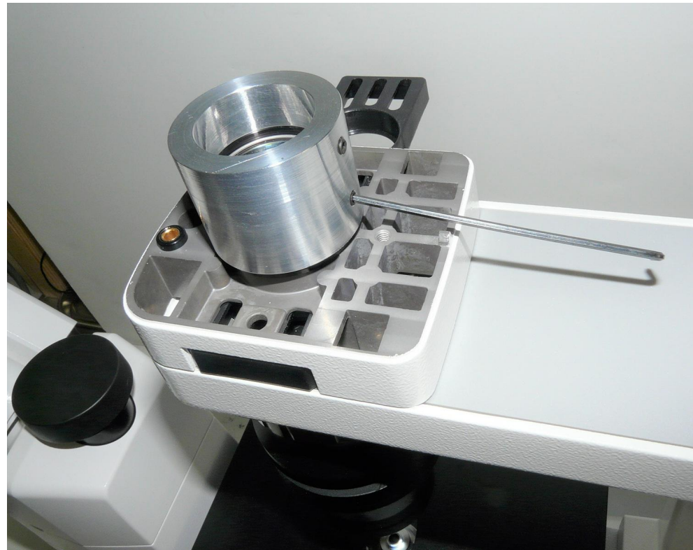
(3) Tighten the set screw using 5/64 in hex key provided.
