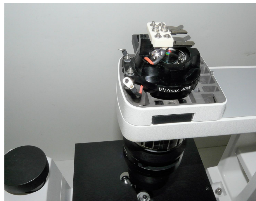
(5) Now ready to remove the original lamp assembly.
