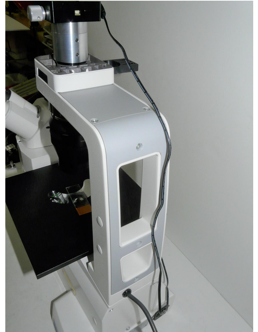
(5) Route the power cable accordingly and now the microscope is ready to operate.
