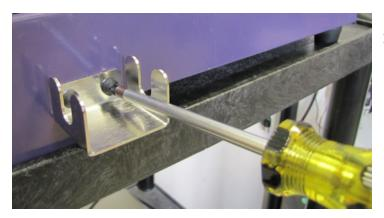
Install the bracket on the right side of the washer to hold the vacuum filtration tubing used to evacuate the filter plate.
