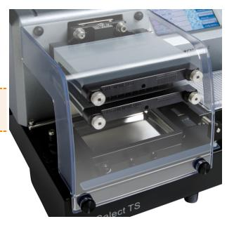
405 LSs equipped with Verify™ Clog Detection Technology ("Q" models) have a smaller mist shield.
