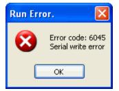
**BioStack** communication error: when controlling the BioStack with the LHC, make sure the onboard configuration setting is **Manual**.
