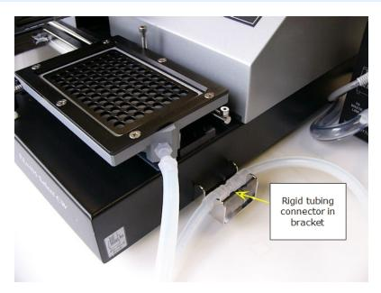
Vacuum Filtration Plate Carrier (and bracket for holding tubing)
