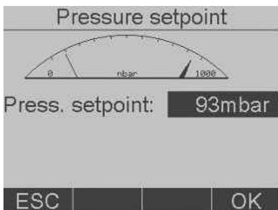
Fig. 6.4: Pressure setpoint with connected Vacuum Pump V-700/710
