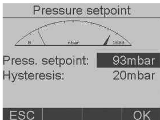
Fig. 6.5: Pressure setpoint without Vacuum Pump V-700/710
