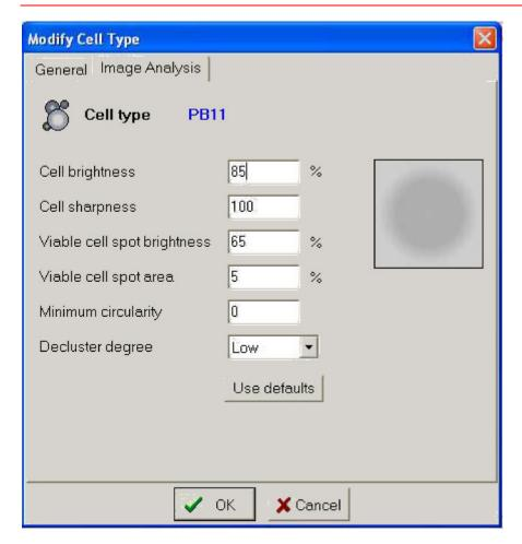
**Cell Brightness:** Is the brightness of the cell boundary within a given image. The range is 50% (darkest) to 90% (lightest). Different cell types will have varying cell 'brightness' settings. The software detects the transition from dark (cell boundary pixels) to light (background of the image). A lower value means a dark boundary will be required for cell identification. A higher value means a lighter boundary.
