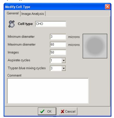
**Minimum Diameter:** The minimum diameter of the cell type. 2 is the minimum diameter allowed. The minimum diameter can be used to exclude debris and/or unwanted cells.
