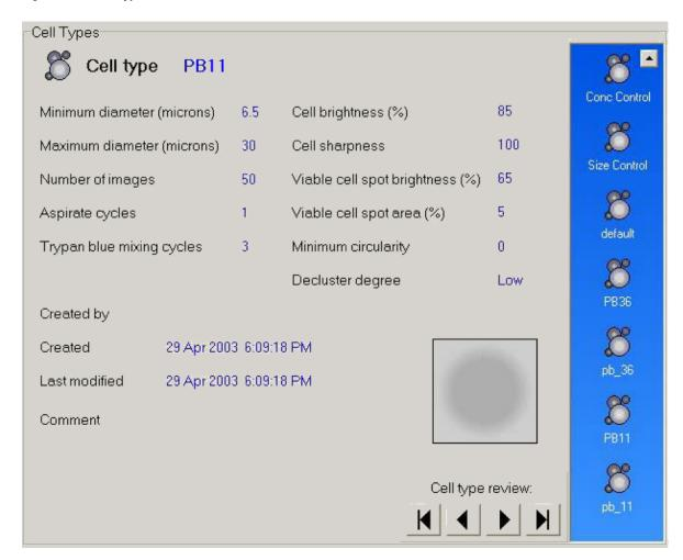
Each cell type provides pre-defined instrument and measurement parameters for ensuring accurate analysis results.
