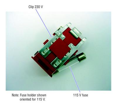
Figure 3.6 Fuse holder and clip and removal of clip
