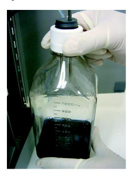
Once reagents have been installed, click on the main screen toolbar, **Instrument** and **Replace reagent pack**. This will prime all lines with reagent and prepare the unit for sample analysis. The reagent level meter will reset to maximum number of runs.
