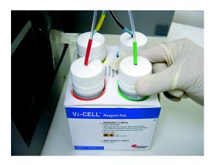
Figure 4.2 Place reagent pack inside the Vi-CELL XR reagent compartment
