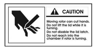
While the CentriVap Concentrator is operating, do not lean on the lid, do not stand near it longer than necessary and do not place hazardous materials within 12 inches.
