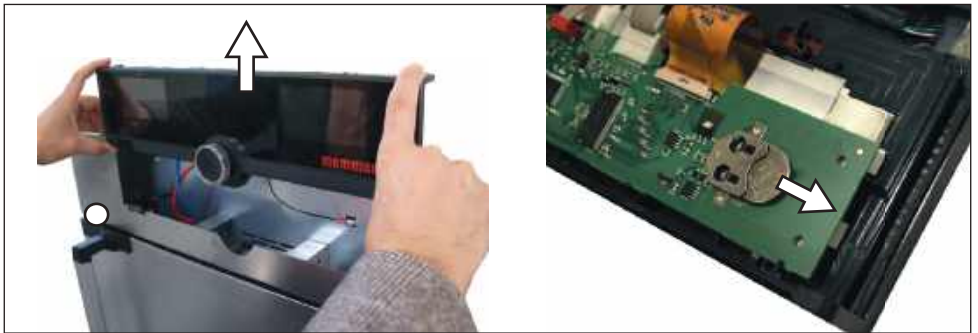
Fig. 34 Removing the lithium battery
