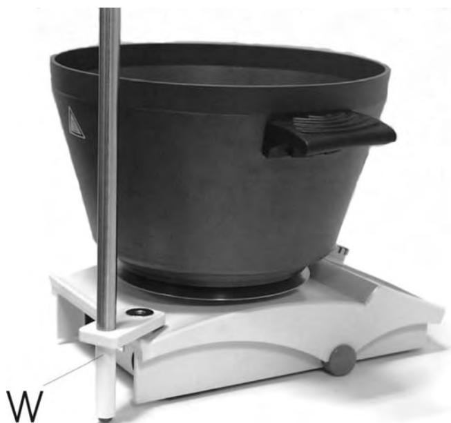
When using the instrument with a heating bath (see Accessories), ensure that the positioning rim on the heating bath is fitted securely over the hotplate.
