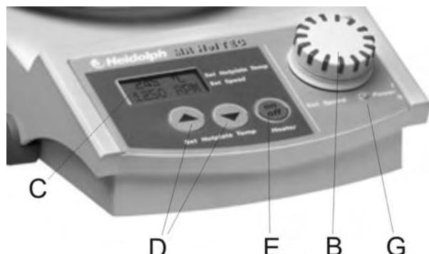
Set the desired speed with the control knob (B). The set speed is shown on the display (C).
