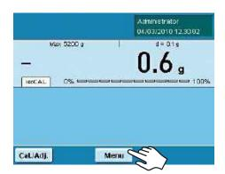
► To open System settings, touch **Menu** when the balance is in the **operating mode**.
