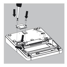
Connect the display and control unit to the electronics module:
