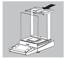
▶ Slide the upper draft shield panel into the guide rails from the rear.
