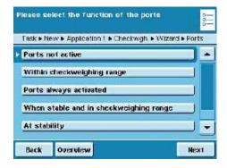
▶ Define how the ports should be activated depending on the check results.
