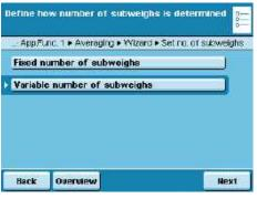
▶ Define the number of measurements to be used for the average value. **Fixed number of subweighs**: You must now enter a fixed number.
