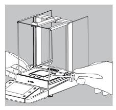
Carefully remove any sample residue/spilled powder using a brush or hand-held vacuum.
