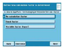
▶ Define whether or not the weighing results should be calculated with an additional factor and how this factor should be applied.
