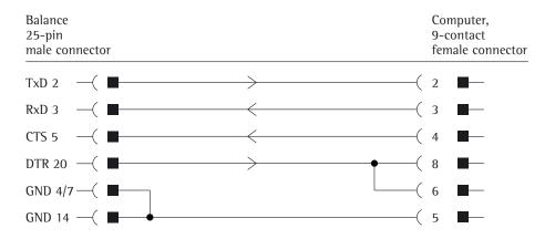
Cable type: AWG 2 specification
