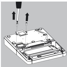
Open the slot for the connection cable on the electronics module:
