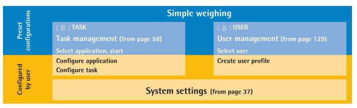
In **Task Management (TASK)**, task profiles with specific applications, weighing and printout settings can be configured.
