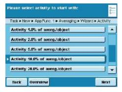
► Enter the sensitivity for the start of the measurement: 0.1%, 0.2%, 0.5% ... \*10% ... 50% of averg./object
