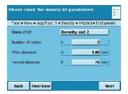
When other vessels or other submersion assemblies are used, this factor can be changed by modifying the parameters for the density kit.
