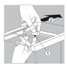
► Slide the upper draft shield panel into the guide rails from the rear while pressing the locking tab.
