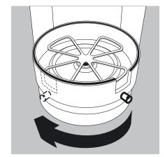
► Turn draft shield parts approx. 90 degrees to the left (loosen knurled screw)
