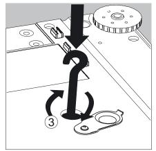
**3.** Carefully screw on the below-balance weighing hook.
