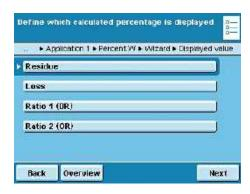
► Define which percent calculation should be used. **Example**: Weight value = 10 g, reference weight = 50 g
