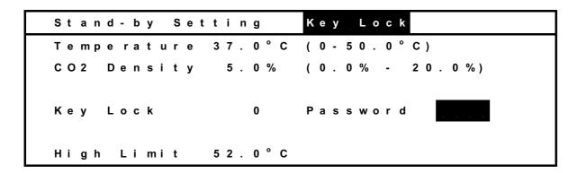
**Note:** The buzzer will sound for a long time if the wrong password is entered. Enter the correct password. The password for releasing the key lock must be shared and administered among all users of the Incubator. The password is set to 0000 when the Incubator is shipped from the factory. The procedure for changing the password is given next.
