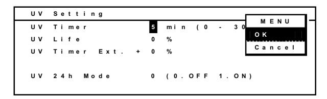
**4.** Press the MENU Key to display the menu, select **OK**, and press the ENTER Key. The parameter will be saved.
