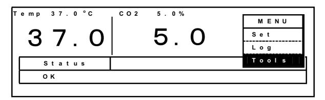
**2.** Select *UV Setting* from the Select Tools Display, press the MENU Key to display the menu, select *OK*, and press the ENTER Key.
