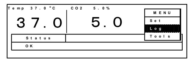
**2.** The log will be displayed with dots. Press the Up Cursor Key and Down Cursor Key to switch between the temperature and CO<sub>2</sub> density displays. Press the Left Cursor Key and Right Cursor Key to scroll the displayed data (Left Cursor Key: older data, Right Cursor Key: newer data).
