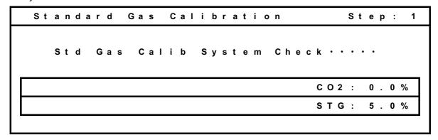
**3.** If the system is normal, the following display will appear. Select OK and press the ENTER Key to start calibrating the  $CO_2$  density. After calibration, return to normal cultivating operation.
