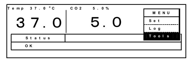
**2.** Select *Date Time* from the Select Tools Display, press the MENU Key to display the menu, select *OK*, and press the ENTER Key.
