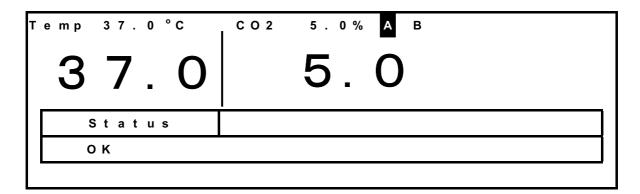
(When the line needs to be switched from cylinder A to B, press the Right Cursor Key for 5 seconds.)
