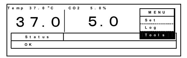
2. Select *Key Lock PW Setting* from the Select Tools Display, press the MENU Key to display the menu, select *OK*, and press the ENTER Key.
