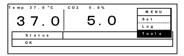
2. Select *Alarm Setting* from the Select Tools Display, press the MENU Key to display the menu, select *OK*, and press the ENTER Key.
