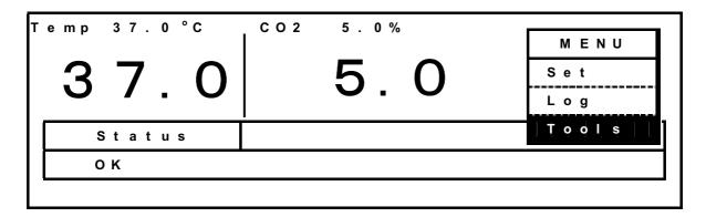
**2.** Select *Temp/CO2 Calibration* from the Select Tools Display, press the MENU Key to display the menu, select *OK*, and press the ENTER Key.
