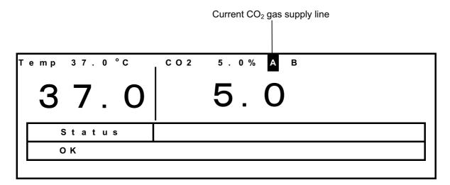
**5.** The MCO-21GC detects that there is no more  $CO_2$  gas in a cylinder when the  $CO_2$  density in the chamber does not increase for a while even after opening the  $CO_2$  gas valve in the Incubator. It switches the gas supply line when it detects that there is no more gas. At that time, the following indications of switching the gas cylinder are provided.
