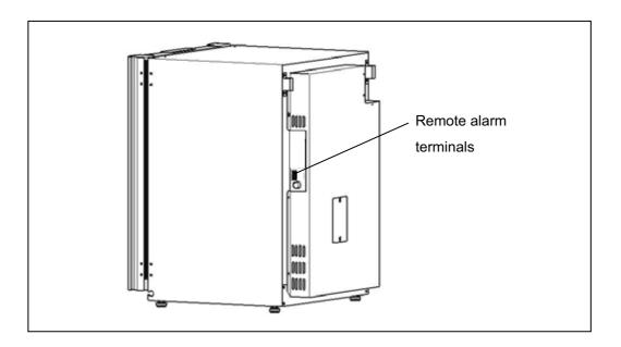
The remote alarm terminals are a contact output.
