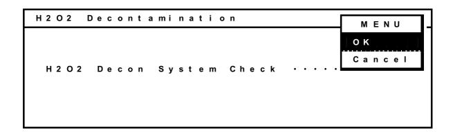
7. If the system is normal, the following display will appear. (If the system is not normal, refer to Table 2 on page 47.) Select OK and press the ENTER Key to start  $H_2O_2$  decontamination. Decontamination will be performed automatically to step 10. The buzzer will sound when decontamination has been completed (It takes about 1 hour 40 minutes after warming-up).
