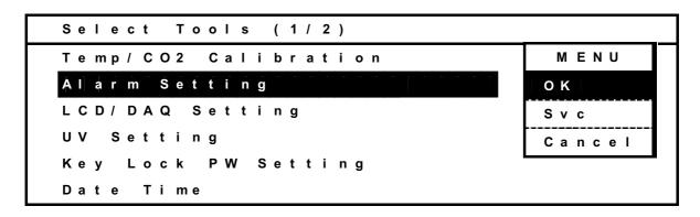
**3.** The Alarm Setting Display will appear. The temperature alarm, CO<sub>2</sub> alarm, alarm delay, ring back time, and door delay can be set on this display. The alarm buzzer can be silenced by pressing the BUZZER Key. The buzzer will sound again after the specified ring back time if the condition that caused the alarm continues. The ring back time can be set.
