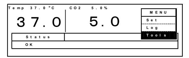
**2.** Press the Down Cursor Key from the Select Tools (1/2) Display to display the Select Tools (2/2) Display, and then select **Standard Gas Setting**, press the MENU Key to display the menu, select **OK**, and press the ENTER Key.
