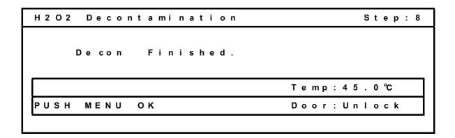
12. Dilute the remaining H<sub>2</sub>O<sub>2</sub> reagent in the H<sub>2</sub>O<sub>2</sub> Generator with a large volume of water and dispose of it. Rinse and wash the H<sub>2</sub>O<sub>2</sub> Generator with distilled water. Then keep the H<sub>2</sub>O<sub>2</sub> Generator in a clean environment outside of the chamber.
