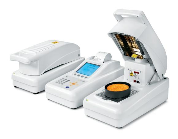
Mark 3 LTE in parallel operation with 2 measuring modules
