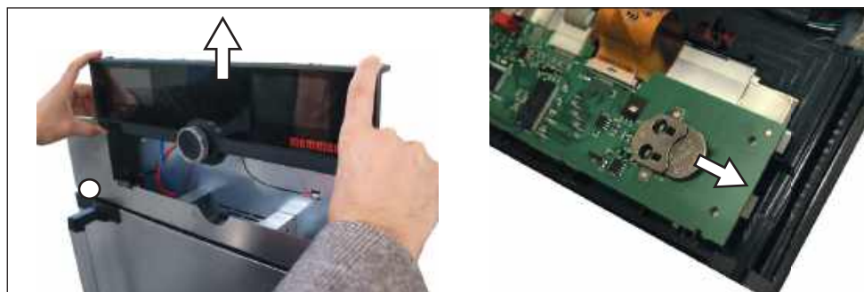
Fig. 25 Removing the lithium battery
