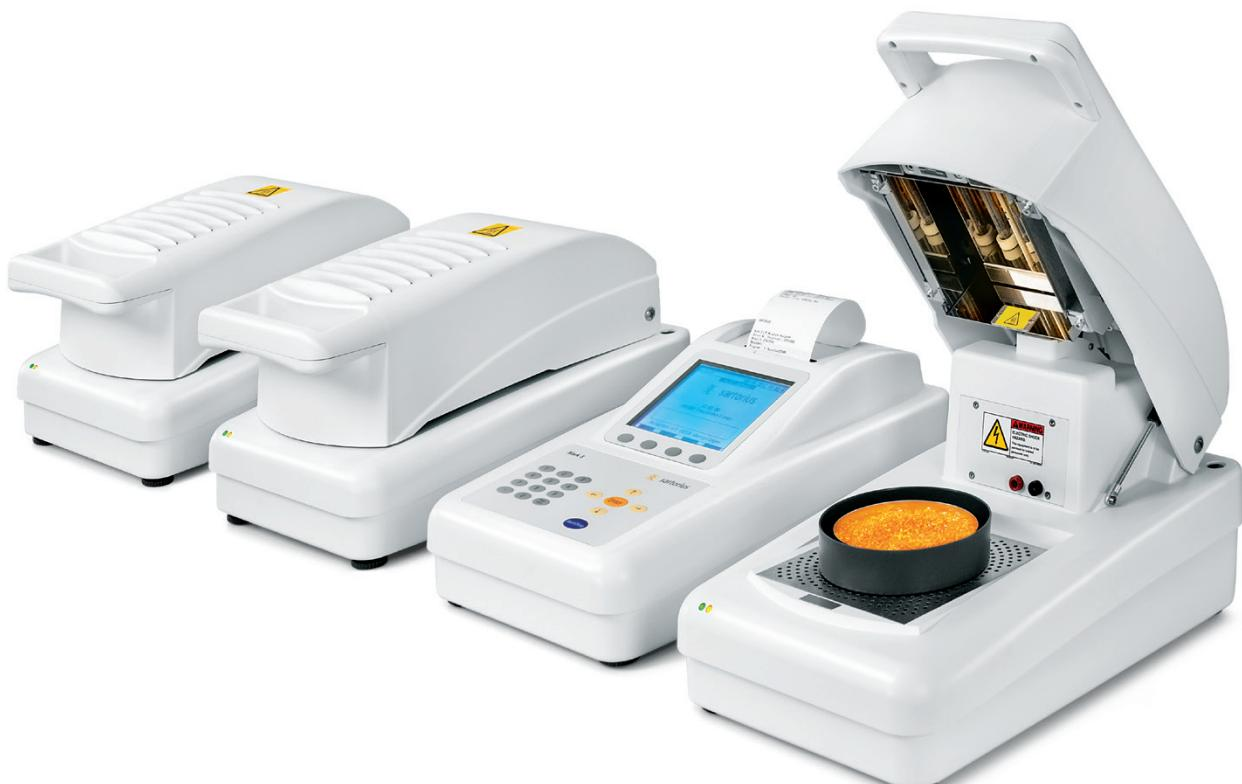
Mark 3 HP in parallel operation with 3 measuring units
