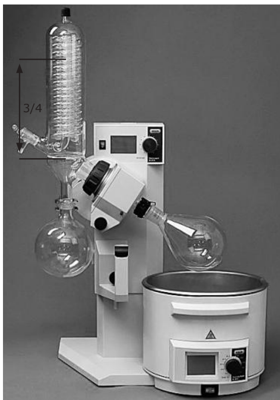
Fig. 6.2: Optional condensation area of a condenser
