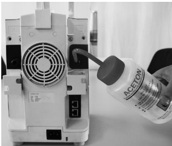
Fig. 7.1: Cleaning the valve head with acetone
