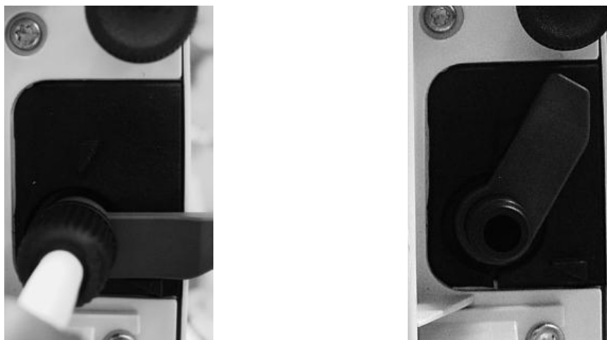
Fig. 4.4: Gas ballast shown open on the picture on the left and closed on the picture on the right
