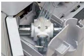
A new type of plunger made with a technique that reflects consideration of the material structure and a precise plunger-holding mechanism help to increase the service life of plunger seals and enable stable solvent delivery over long periods.
