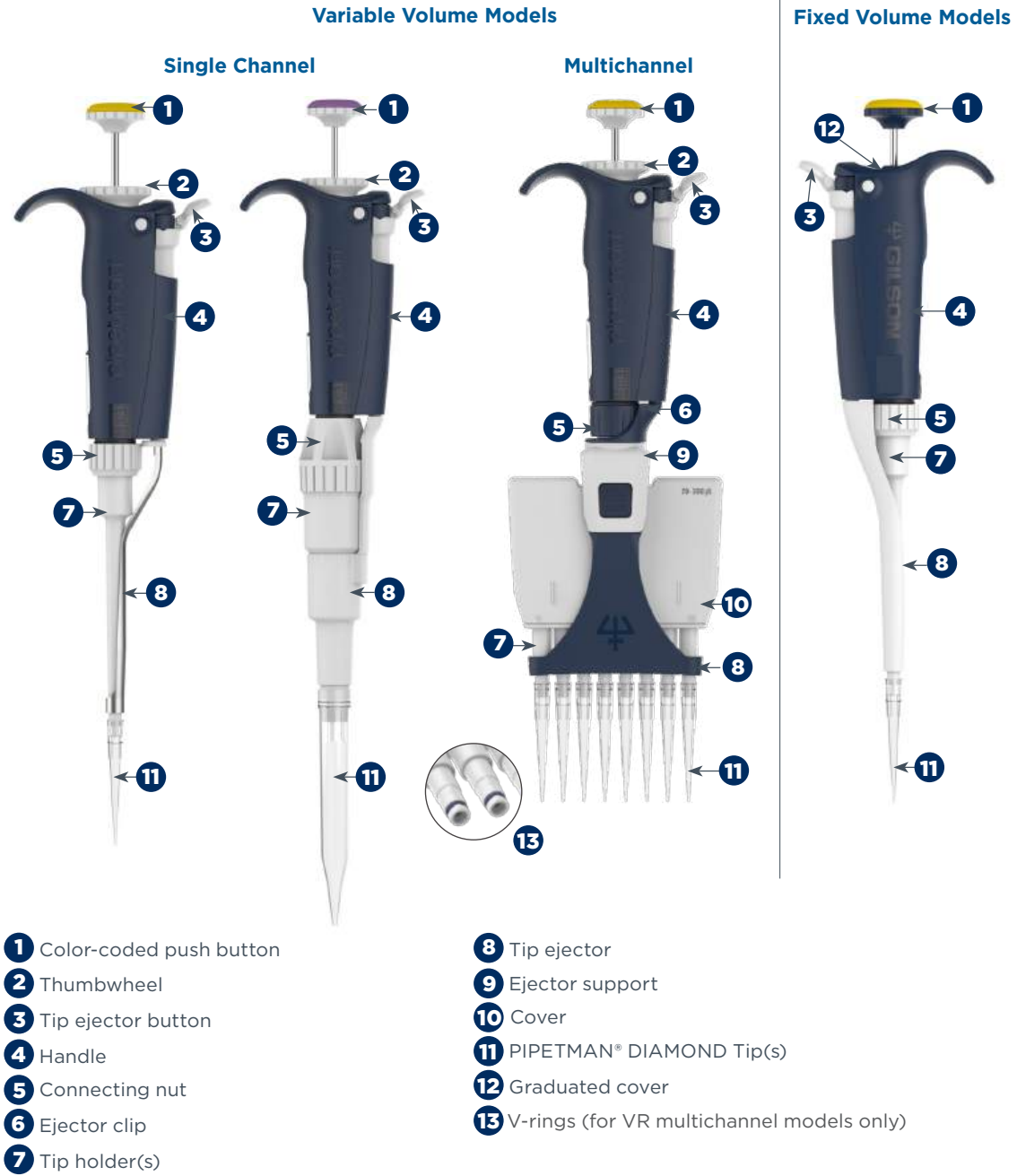
Figure 2 PIPETMAN® L single channel, multichannel, VR multichannel, and fixed volume model components
