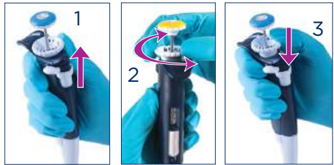
Figure 5 Volume unlock and lock
