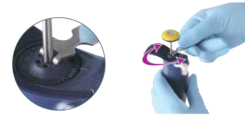
Figure 6 PIPETMAN® L fixed volume model adjustment—hold the key in the highest position to avoid banging it into the hook
