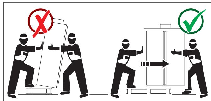
When the cabinet touches the ground, support it so that the pallet can be removed.
