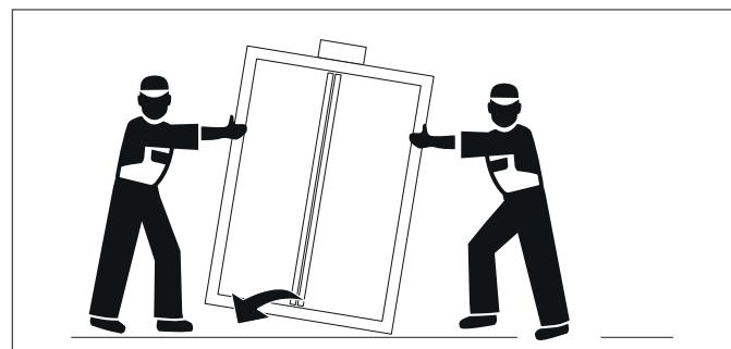
After installing the cabinet, remove the protections for
