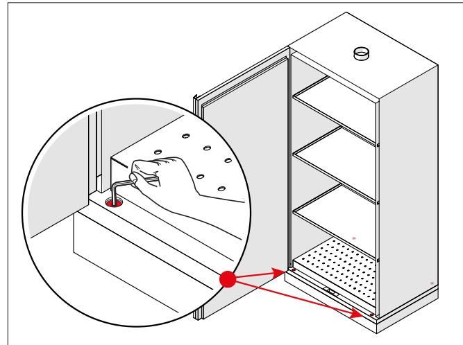
**⚠** During the opening and closing phases, the door elements must not slide over the fire-protection seals near the door stops. Doors equipped with automatic closing system must close automatically from any position and the lock must be lockable.
