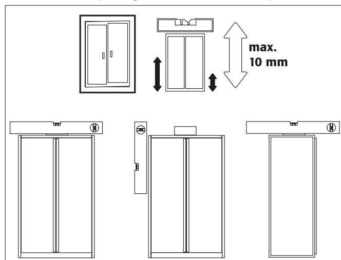
If necessary, level the cabinet by adjusting the support feet.
