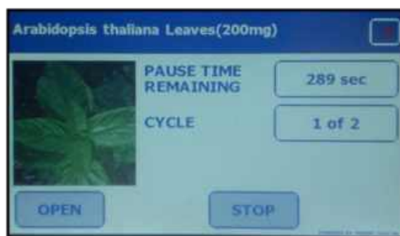
Figure V-7: FastPrep-24™ 5G ‘Touch Screen’ Countdown Display During Cycle Pause
