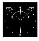
With the aid of METTLER DeltaTrac you can check fill quantities and determine deviations from a definable target weight in percent.
