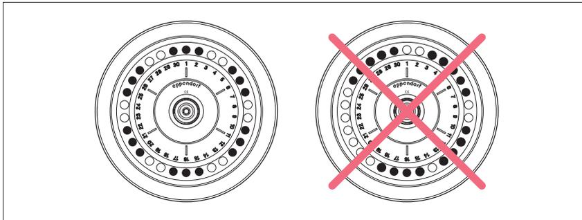
To keep the weight differences between the filled sample tubes low, we recommend taring with a balance. This protects the drive and reduces operating noise.
