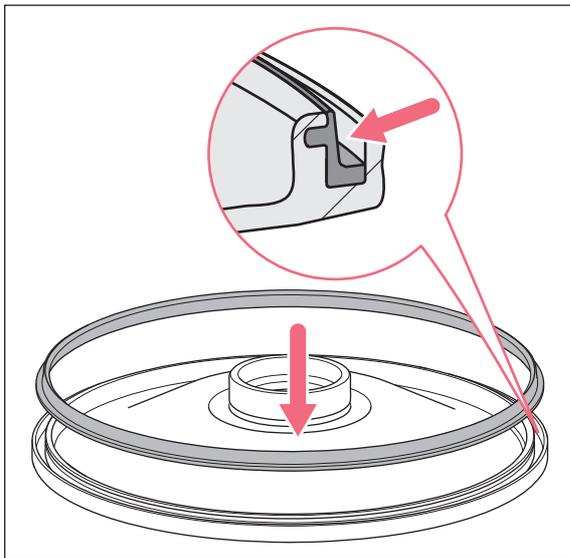
5. Insert the sealing ring in the clean groove of the rotor lid.
