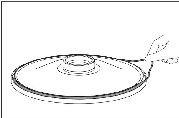
1. Remove the sealing ring to thoroughly clean the groove below it.
