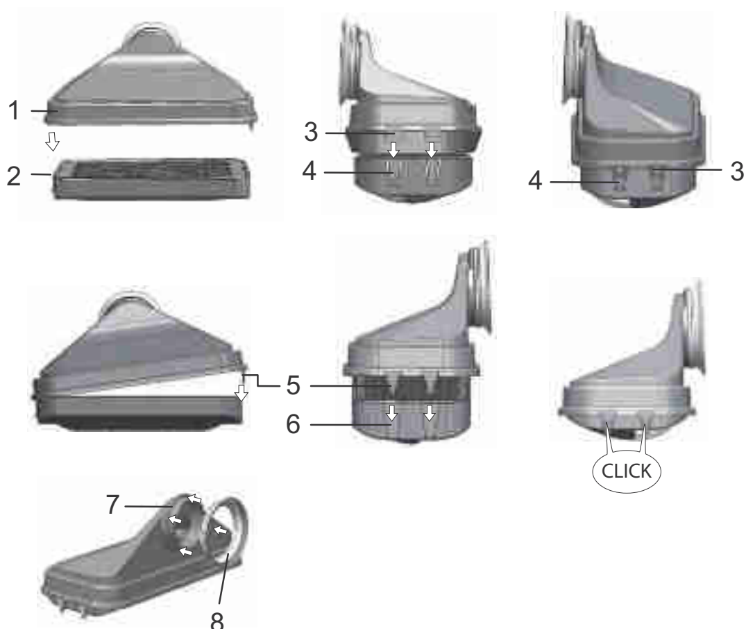
Figure 4-4. Assembling the HEPA-filter and the airbox
