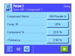
When defining specifications for the individual components, a **percentage nominal value** must be entered instead of an absolute nominal weight (depending on the selected "**Basis**", this refers to either the total weight of the formula or the first component).
