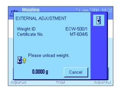
Once the requested weight is placed on the pan, the adjustment operation is carried out automatically. At the end of the adjustment operation you are prompted to lift off the weight. Remove the adjustment weight from the weighing pan.
