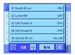
The example opposite shows the first page of the component database with the first five components.
