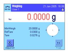
Press the  $<\!\!\!\!<\!\!\!> 0 \leftarrow\!\!\!\!>$  key to set the display to zero. Place the tare (weighing container) on the weighing pan and press the  $<\!\!\!> 1 \leftarrow\!\!\!>$  key to tare the balance. The balance determines the tare value and displays it in the "Tare" information field. The "Net" icon (net weight) appears next to the weight display.
