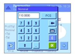
Press the "Nominal" function key. Type in the desired value. Check the weighing unit, which is shown to the right of the nominal value. When the weighing unit is touched a selection box containing the available units, including "PCS" (Pieces), appears. Note: The "PCS" unit is available only if a reference piece weight has been determined. The units are not converted automatically; i.e., if a value is entered in one unit, this value remains the same even if the weighing unit is changed.
