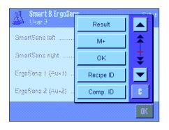
"Result" and "M+" emulate the function keys of the same name. "OK" emulates pressing the button of the same name in the formulation dialog boxes (but not in the menus) to confirm entries and actions.
