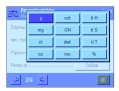
In the menu for the "Display Unit" and the "Info Unit", in addition to the known weighing units the unit "%" (percent) is available (provided that a reference has already been determined).
