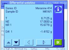
You can use the "Info" function key at any time to display the results of differential weighing. In the example opposite, the results for the first sample are displayed (press the arrow key at the bottom right of the screen to display the results of further samples). The values have the following meaning:
