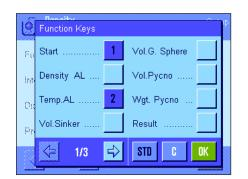
"Start": This is the function key you use to start the density determination, so it must always be activated!
