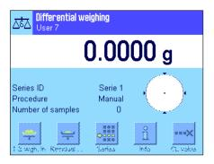
When the application has been selected, the display opposite appears. Some of the specific function keys, as well as specific information fields for differential weighing, are activated ex works. You can adapt these and other settings to your own requirements, as described in the following sections.
