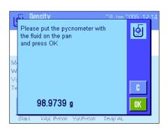
Press the "Start", function key to start the density determination. You will then be prompted to place the filled pycnometer (the selected weight of the pycnometer appears in the lower left-hand corner of the window with a minus sign).
