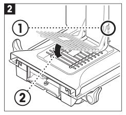
Insert the grid weighing pan from the front.
