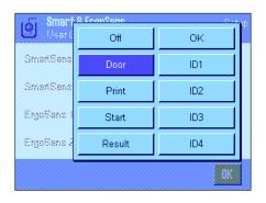
"Start" and "Result" emulate the function keys with the same names. "OK" emulates pressing the key with the same name in the density determination dialogs (but not in the menus) to confirm inputs and actions.
