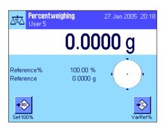
After you have selected the application, the display shown at left appears. Some of the special function keys and the special information fields for percent weighing are activated at the factory. How you can adapt these and other settings to your needs is described in the Sections that follow.
