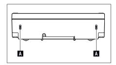
To change the reading angle, press in the two buttons (A) on the back of the terminal. The top of the terminal can then be pulled up or down until it engages in the desired position. A total of 3 setting positions are available.
