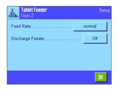
"Feed Rate": Select the desired feed rate: "slow", "normal", "fast" or "very fast".
