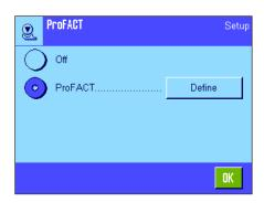
The settings for fully automatic adjustment are defined in this menu using the **internal** adjustment weight (ProFACT). ProFACT (**Pro**fessional **F**ully **A**utomatic **C**alibration **T**echnology) provides fully automatic balance adjustment based on preselected time and/or temperature criteria.
