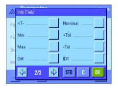
"Min" and "Max": Smallest and largest recorded piece counts in a series of piece
