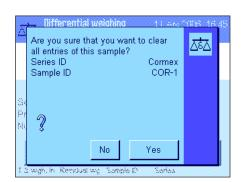
Before deletion, the balance requires you to confirm that you actually want to delete all values for the selected sample. When you confirm the prompt, all available values for tare, weighing in and residual weighing are deleted, and the sample ID is reset to the factory default setting. Check the ID before continuing to work with this sample.
