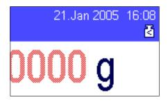
In the illustration opposite, the small **weight icon** above the weighing result (status icon) and the **gray** color of the weight value indicate that the minimum initial weight value has not yet been reached and that the current weight value may be outside the tolerance range specified in the QA system.
