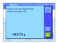
After you have tared the sinker you are prompted to pour the liquid whose density you want to determine into a container. If you are working with the optional density kit, follow the instructions supplied with the kit. If you are working with the below-the-balance hanger, place the container with the liquid under the hanger.
