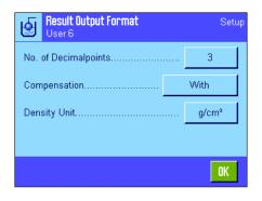
"No. of Dec. Points": The result of the density determination can be displayed and
