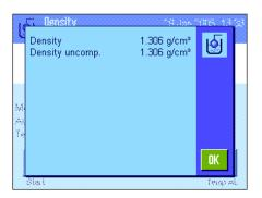
The balance now determines the density of the solid body and displays the result. Either the compensated result, the uncompensated result, or both is/are displayed depending on the settings you made for the result display (see Section 12.3.5).
