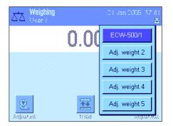
A list for selecting the adjustment weight will appear when you press the function key "Adjust. ext.". **Note**: All adjustment weights in the figure shown here still have the names they were given at the factory, with the exception of the first weight, which was assigned a unique name (Section 5.3.4). The adjustment starts immediately after the weight is selected
