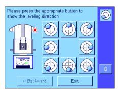
Watch the level indicator on your balance (this will light up when the level sensor is switched on) and press the button that matches the current position of the air bubble in the level indicator.
