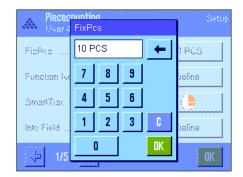
This menu can be used to assign a fixed reference piece number to the "FixPcs" function key (Section 10.3.3). After pressing the corresponding button, an input window appears in which you can define the desired reference piece number.
