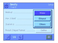
"Water": The density of distilled water at temperatures from 10.0°C to
