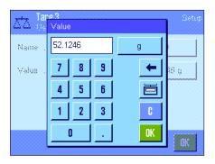
To enter the weight value, press the corresponding button. A numeric input field appears, in which the tare value can be entered. **Note:** Instead of typing in the value, you can place the relevant tare container on the weighing pan and then press the button with the balance icon. The measured weight value is thus transferred directly. Notes on working with the tare memories can be found in Section 7.3.2.
