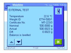
Pressing this function key checks that your balance was adjusted correctly using an external weight. This can be implemented at any time.
