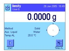
In the application-specific settings, select the method for "**Solid**" (Section 12.3.2) and specify the desired auxiliary liquid (Section 12.3.3).
