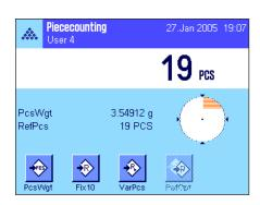
Proceed with the piece count, and place additional pieces on the weighing pan. To optimize the reference, press the "**Ref.Opt**" function key. The number of pieces in the pan is now used as the new reference piece number and the reference piece weight is recalculated on this basis.
