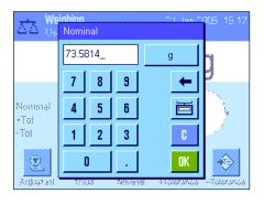
The "+Tol" and "-Tol" function keys can be used to specify the accuracy with which you wish to weigh. The input window is the same as for the nominal value. The input window is the same as for the nominal value. Both tolerance values are set to 2.5% ex works. Instead of a percentage value, you can also enter an absolute tolerance in any weighing unit (e.g., "g"). Once the relevant value is entered, press "OK" to activate the tolerance.
