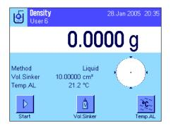
In the application-specific settings for the method, select "**Liquid**" (Section 12.3.2).
