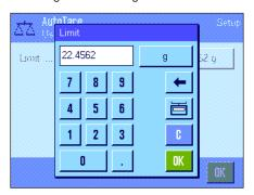
When you activate the "AutoTare" function ("On"), press the button to define the weight criterion for the automatic tare function:
