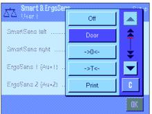
Each of the 4 sensors can be assigned one of the following functions by touching the relevant button:
