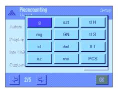
In addition to the common weighing units, the menus for the "Display Unit" and the "Info Unit" also contain the "PCS" unit (provided that a reference piece weight was already determined).
