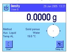
In the application-specific settings, select "**Solid porous**" as your method (Section 12.3.2), and specify the desired auxiliary liquid (Section 12.3.3).
