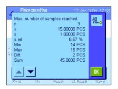
The results window contains the results of the counting series (the information selected for printing the result is displayed, see Section 10.3.7). Please refer to the notes in Section 10.4.5 regarding the units, resolution and accuracy of displayed values.
