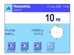
Determine the reference using the desired method (fixed or variable reference piece number, see Section 10.4.1). A reference piece number of 10 is used in the example opposite.
