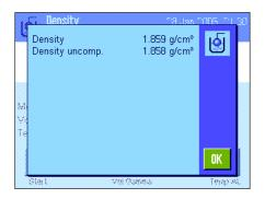
The balance now determines the density of the pasty substance and displays the result. Either the compensated result, the uncompensated result, or both is/are displayed depending on the settings you made for the result display (see Section 12.3.5).
