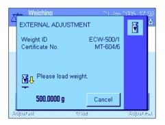
After the adjustment process starts, you will be prompted to place the adjustment weight. If available, the ID and the certificate number of the corresponding weight are displayed. The required weight value flashes at the bottom of the window.
