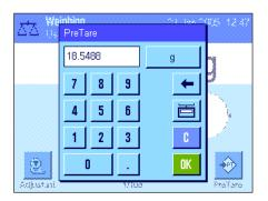
Type in the desired tare value. Check the weighing unit, which is shown to the right of the tare value (custom weighing units are not available when the tare value is entered manually).
