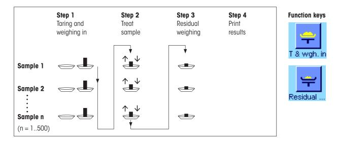
**Method 2** (with separate taring and weighing in)
