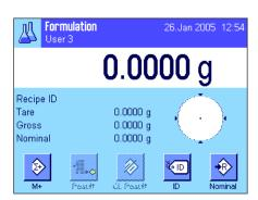
The display opposite appears when the application is selected. The special function keys and information fields for formulation are activated ex works. These and other settings can be adapted to your requirements, according to the descriptions in the following Sections.
