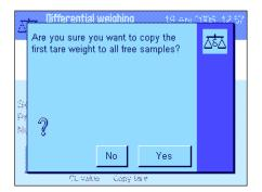
When the function key is pressed, the prompt opposite appears. When you respond with yes, the tare weight of the first sample is copied for all further samples in the current series (as long as no tare weight has already been defined for these samples).
