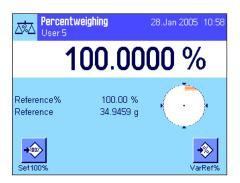
If the reference weight placed on the pan should equal 100%, press the function key for "Set100%" .
