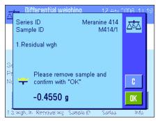
When residual weighing is complete, you are prompted to remove the sample. Remove the sample vessel containing the sample and confirm with "OK".
