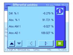
If the results for one sample take up several windows, you can use the scroll buttons at the bottom left of the screen to switch between the individual results windows.
