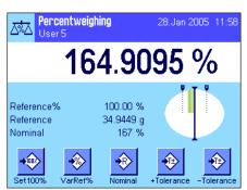
When you have input the target value and the tolerances, tolerance marks for the graphical weighing aid ("SmartTrac") appear in the display. The tolerance marks make weighing to the target value easier for you. You can weigh your weighing sample roughly until the lower tolerance value is reached, and then if necessary dispense finely until the target value is reached.
