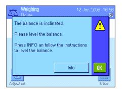
When the level sensor detects that the level is incorrect, the warning text at left will appear and a warning beep will sound. A status icon will also appear in the upper right-hand corner of the display (below the time).
