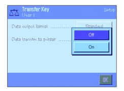
When you press the "**Transfer**" function key, the data are normally only transmitted to the host. If you also want to send the data to the printer, activate the setting "**Data transfer to printer**". **Note**: The previously described settings for formatting the data do not affect how the data is output to the printer. This is entirely controlled by the protocol settings (Section 7.2.8).
