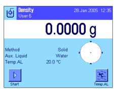
When you have selected the application, the display shown at left appears. Special function keys and information fields for density determination are activated at the factory. The balance is preset to use water as the auxiliary liquid for density determination. However, you can change these settings according to your needs as described in the Sections that now follow.
