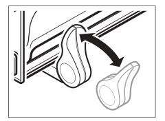
For **motorized door operation** the handles must be connected:
