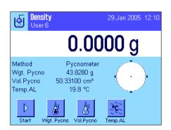
In the application-specific settings, select "**Pycnometer**" as your method (Section 12.3.2).
