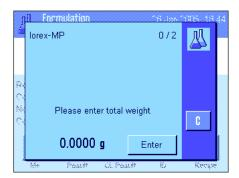
Depending on the basis for weighing in components, which is specified in the formula definition (Section 9.5.2), when the formula is called up you will first be prompted to enter the desired **final weight of the formula** or the **nominal weight of the first component**. Enter the required value.
