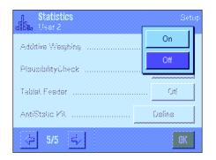
**"On":** Additive mode is switched on. Following manual or automatic transfer
