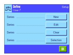
Press the «== » key and select the menu for defining a series (on the first menu page). This menu contains options for creating a new series, and for editing or deleting an existing series. In the final menu option, you can select the series with which you want to work. These options are explained in more detail in the following sections.
