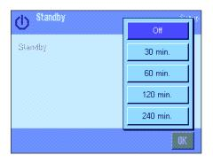
You can switch off standby mode ("Off") or define a time of 30, 60, 120 or 240 minutes, after which the balance should enter "Standby" mode. "Standby" mode is the same state that the balance enters if it is switched off using the «**On/Off**» key. Press the «**On/Off**» key to switch the balance on again.
