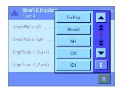
"FixPcs", "Result" and "M+" emulate the function keys of the same name. "OK" emulates pressing the button of the same name in the piece counting dialog boxes (but not in the menus) to confirm entries and actions.
