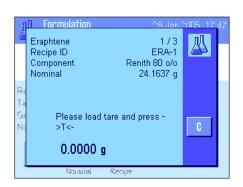
You will be prompted to tare the balance. Place the weighing container on the balance and press the  $*\rightarrow$ **T** $\leftarrow$ » key.
