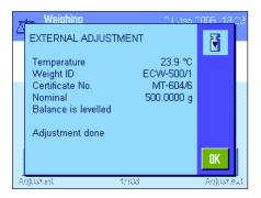
The balance confirms that adjustment was carried out successfully. Press "**OK**" to return to the application.
