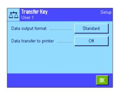
You can use the "**Transfer**" function key to transmit the stable weight value across the interface to a host computer (Section 7.2.2). In this menu you can specify how you want the output values to be formatted. You may need to do this if you use your balance together with other instruments, programs, or peripheral devices that require a particular data format. You can also use this menu to specify whether the data should only be output to the host or also to the printer.
