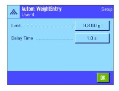
When you activate this function ("On"), press "Define" to define the criteria for automatic weight transfer:
