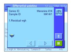
The balance displays the first sample in the series for which no corresponding residual weight values are available. If you want to perform residual weighing for a different sample, press the arrow key at the bottom of the window. In this example, however, we presume that you want to start with the first sample. Confirm this by pressing "**OK**".
