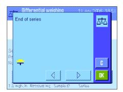
After the last sample, a message is displayed confirming that taring and weighing is complete for all samples in the series.
