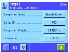
In this menu window, first select the desired component from the component database and then define its nominal weight and the permissible tolerances.
