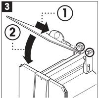
Insert the top door of the draft shield at an angle (slightly less than 30 degrees) into the guide positioned at the back, and swivel the draft-shield door carefully down (see Fig. 3).
