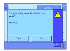
Choose "Series....Clear". A selection field is displayed in which you can select the series that you want to delete. Before the series is deleted, the prompt displayed opposite appears. If you respond with yes, the series is deleted together with all measured values and calculated results.
