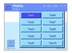
When the "Tare Store" function key is pressed, a window appears in which you can select the desired tare memory. The memory names correspond to those that were defined in the menu ("Tare 1"..."Tare 10" are only example names).
