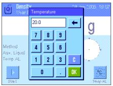
If you use **water or ethanol as the auxiliary liquid**, enter its **temperature** with the "**Temp. AL**" function key. (Density tables for these two liquids in the temperature range 10 °C to 30°C are stored in the balance, see also Sections 12.7 and 12.8). The screenshot at left shows the corresponding input field (input in °C with one decimal place).
