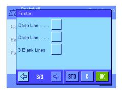
This submenu can be used to define the information to be printed at the bottom of the weighing record after the results (single values). The footer is printed when the "Footer" function key is pressed. The footer options are the same as those for the header, only the "Levelcontrol" option is unavailable.
