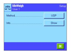
If the "MinWeigh" function has been enabled, it can be activated or deactivated in the menu. When the function is activated, press "Define". The following options are available:
