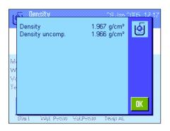
The balance now determines the density of the liquid and displays the result. Either the compensated result, the uncompensated result, or both is/are displayed depending on the settings you made for the result display (see Section 12.3.5).
