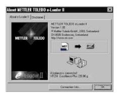
Before you update the software of your balance, please check in the "Help" menu that the communication with the balance is functioning. (In the example shown here, the e-Loader II is confirming that a balance is connected.)
