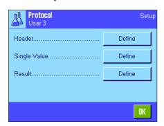
The three submenus for defining the record header, printing single values and for the result contain additional settings for the Formulation, which are described below.
