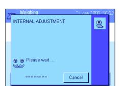
As soon as the preselected time and/or temperature criterion is met (Section 5.3.2), the small ProFACT icon appears in the top right corner of the display, below the time. The balance uses this to indicate that it wishes to carry out a ProFACT adjustment.
