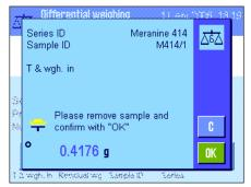
Once weighing in is complete, you are prompted to remove the sample. Remove the sample vessel containing the sample and confirm with "**OK**".
