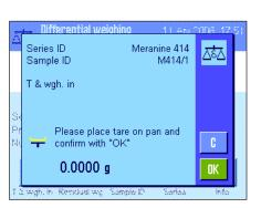
Wait until the balance prompts you to load the weighing vessel (tare) for the first sample. When you have done this, press  ${}^{\circ}$ **OK**''. While the balance is determining the tare weight, a corresponding message is displayed.
