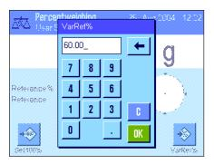
If, instead, you want to make the weight on the pan a **variable reference**, press the function key for "**VarRef%**". An input field appears in which you can specify the percentage value (e.g. 60%) which the weight on the pan should represent.
