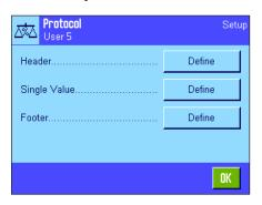
In the three submenus where you can specify the options for the header line of the report, for reporting the individual values, and for the footer line, you also have additional settings available for percent weighing which are described below.
