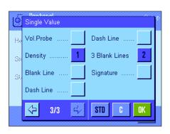
"Vol. Probe": Reports the volume of the sample (which is calculated by the
