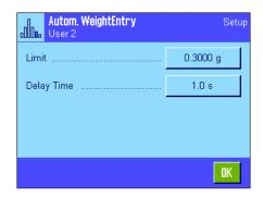
When you activate this function ("On"), press "Define" to define the criteria for automatic weight transfer:
