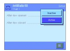
Here you can define whether ionization will occur when the glass draft shield is opened ("Active") or whether no ionization will occur ("Inactive"). With the "Active" setting, ionization will occur continuously until the doors are closed again (a maximum of 10 minutes).
