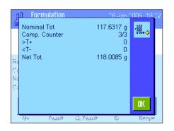
Once all the components of the formula have been weighed in, the window with the results of the formulation appears automatically (the information selected for printing the result is displayed, see Section 9.3.5). The formula record is closed simultaneously (a complete sample printout can be found in Section 9.6.5).
