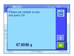
Press the "**Start**" function key to start the density determination. You are then prompted to place the sample on the balance (without the gamma sphere).
