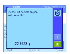
Press the "**Start**" function key to start the density determination. The balance executes an automatic tare and you will then be prompted to place the solid body on the balance to weigh it in air.
