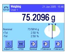
As soon as the nominal value and tolerances have been entered, a graphic weighing-in aid ("SmartTrac") appears in the display with tolerance markers that simplify weighing in to the nominal value: You can roughly weigh in your samples until the lower tolerance value is reached and then accurately dose, if necessary, up to the nominal value.
