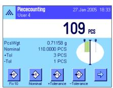
As soon as the nominal value and tolerances have been entered, a graphic weighing-in aid ("SmartTrac") appears in the display with tolerance markers that simplify weighing in to the nominal value: You can roughly weigh in your samples until the lower tolerance value is reached and then accurately dose, if necessary, up to the nominal value.
