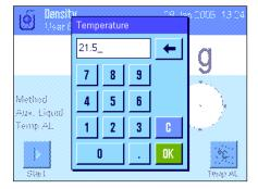
If you are using **water or ethanol as the auxiliary liquid**, enter its **temperature** using the "**Temp. AL**" function key. Density tables for these two substances covering the temperature range from  $10\,^{\circ}\text{C}$  to  $30\,^{\circ}\text{C}$  are stored in the balance; see also Sections 12.7 and 12.8). The illustration here shows the corresponding input field (input in °C with 1 decimal figure).
