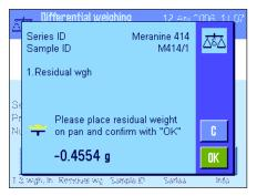
Wait until the balance prompts you to load the selected sample for residual weighing. Load the weighing vessel (tare) with the first sample and then press  $\mathbf{\tilde{O}K}''$ .
