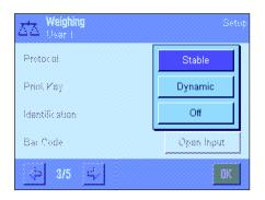
"Stable": When the «🕮» key is pressed, the record is not printed until the
