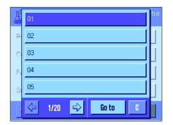
Press the «== » key and select the menu for defining components (on the first menu page). The first page of the component database appears. The database comprises a total of 20 pages with 5 components on each. The arrow keys can be used to switch between the individual pages. Each of the 100 components can be selected directly by pressing the "Go to" button and entering the component number. In the illustration opposite, the database does not yet contain any entries.
