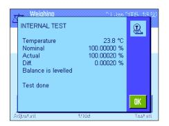
Following successful completion of the test, the window opposite is displayed as confirmation. If a printer is connected to the balance, the test is printed automatically according to the specifications selected in the system settings for printing (Section 5.3.7). A sample printout can be found in Section 7.4.6.
