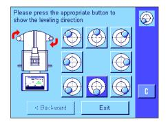
The Leveling Assistant will show you with red arrows which direction you need to turn the two footscrews on the back of the balance.
