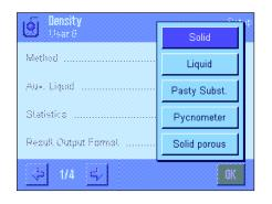
**"Solid":** Density determination of non-porous solid bodies using an auxiliary
