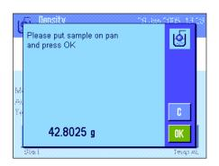
Press the "**Start**" function key to start the density determination. The balance will automatically carry out a taring, after which you will be prompted to put the solid in place (first weighing in air).
