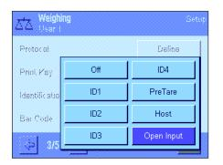
"Off": No bar code data is processed. This setting should be used if no
