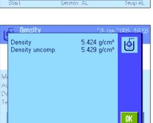
The weighing result is saved and you are then prompted to immerse the solid body in the auxiliary liquid.
