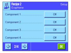
Menu pages 2 to 4 can be used to select components, which are to be part of the current formula and to define specifications for their processing. All components are deactivated ex works ("Off").
