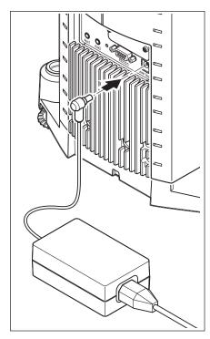
Your balance is delivered complete with an AC adapter and a country-specific power supply cable. The AC adapter is suitable for all power supply voltages in the range:
