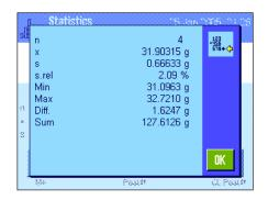
The results window contains the results of the weighing series (the information selected for printing the result is displayed, see Section 8.3.5). Please refer to the notes in Section 8.4.3 regarding the units, resolution and accuracy of displayed values.
