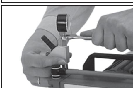
Assemble control valve first, then align and fasten gauge.
