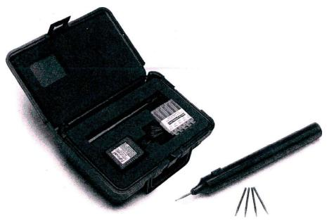
WARNING: For research use only. Not for use on humans. The Ideal Micro-Drill™ is designed for research applications that - require burrs and trephines. The drill is constructed of light-weight aluminum alloy for balance and control and is powered by a rechargeable 6-volt nickel-metal hydride (NiMH) battery. Under normal operating conditions and with intermittent use, the unit will work for up to 8 hours on a full charge.
