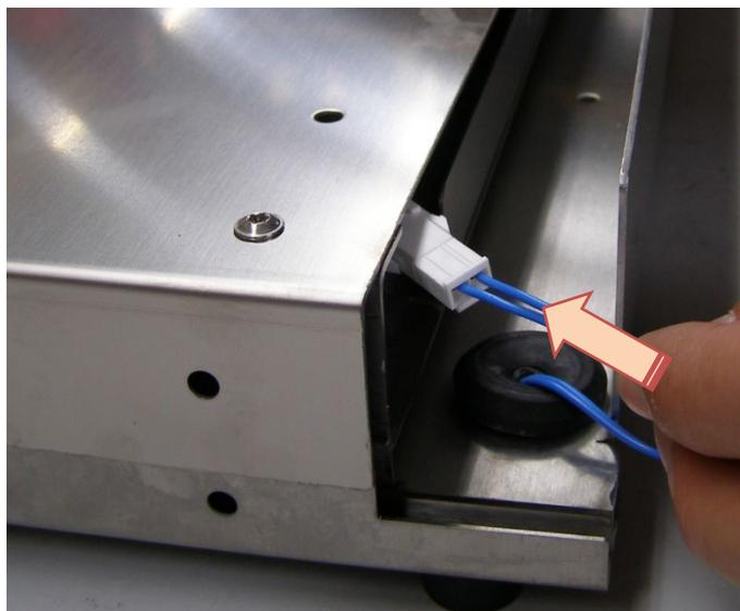
Slot the back panel ② onto the base ①. The connecting link of the base ① must fit in the back panel ②. **Take care not to squeeze the sensor cable.**
