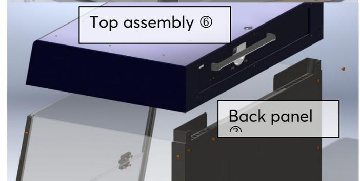
Connect the sensor cables from the back panel ② and the top assembly ⑥. Put the power plug of the back panel ② into the power outlet of the top assembly ⑥.
