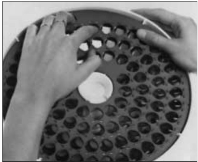
Fig. 10. Snapping the tube holder into place.
