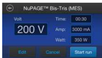
Figure 8 Pre-programmed Method for NuPAGE™ Bis-Tris Mini Gels
