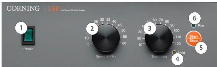
1. **POWER switch:** Turns the shaker ON (power switch illuminates) or OFF
