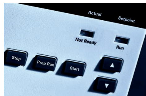
Simple 5-button keypad minimizes the chance of operator errors.
