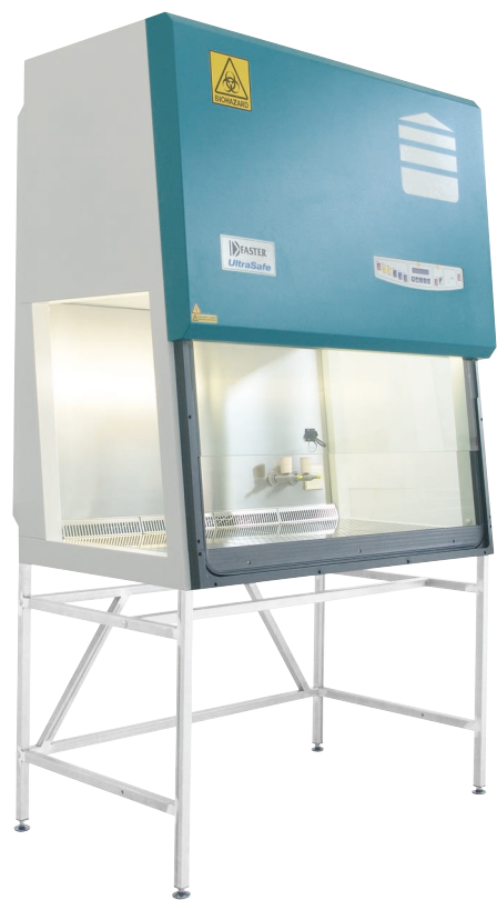
Faster UltraSafe cabinet features an ergonomically angled sloping-front, fitted with electrically operated vertically sliding safety-glass sash window, the framework of which is also hinged and can be opened up for easy access during cleaning and maintenance.
