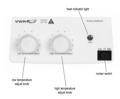
These multi-purpose units are ideal for incubation and activation of cultures, enzyme reactions, immunoassays, melting/boiling points and a wide variety of other laboratory procedures.
