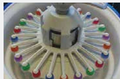
QuickPrep™ 3 Adapter 24 x 2 mL tubes (included with FastPrep-24™ 5G instrument) Cat. No. MP116005512
