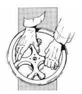
**b.** Tighten the tie-down screw clockwise onto the drive shaft.
