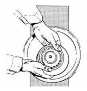
**b.** Tighten the tie-down screw clockwise onto the drive shaft.
