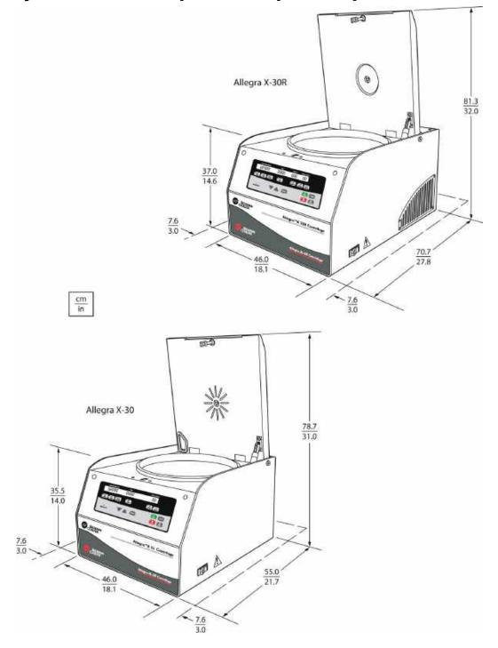
Figure 4.1 Dimensions of the Refrigerated and Nonrefrigerated Centrifuges
