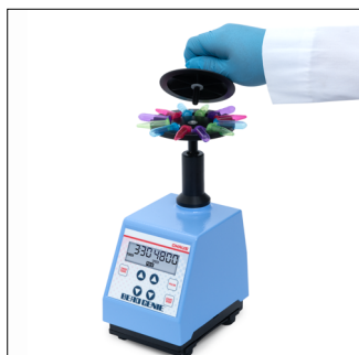
4. Put lid on and tighten thumbscrew
