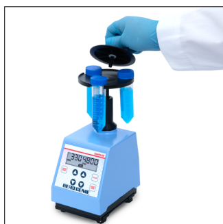
4. Put lid on and tighten thumbscrew
