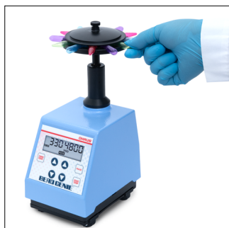
5. Check if tubes are firmly clamped
