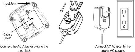
Battery installation (without optional internal battery):
